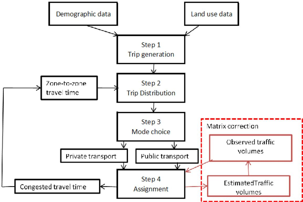
**Figure 8. 4-step model scheme**
