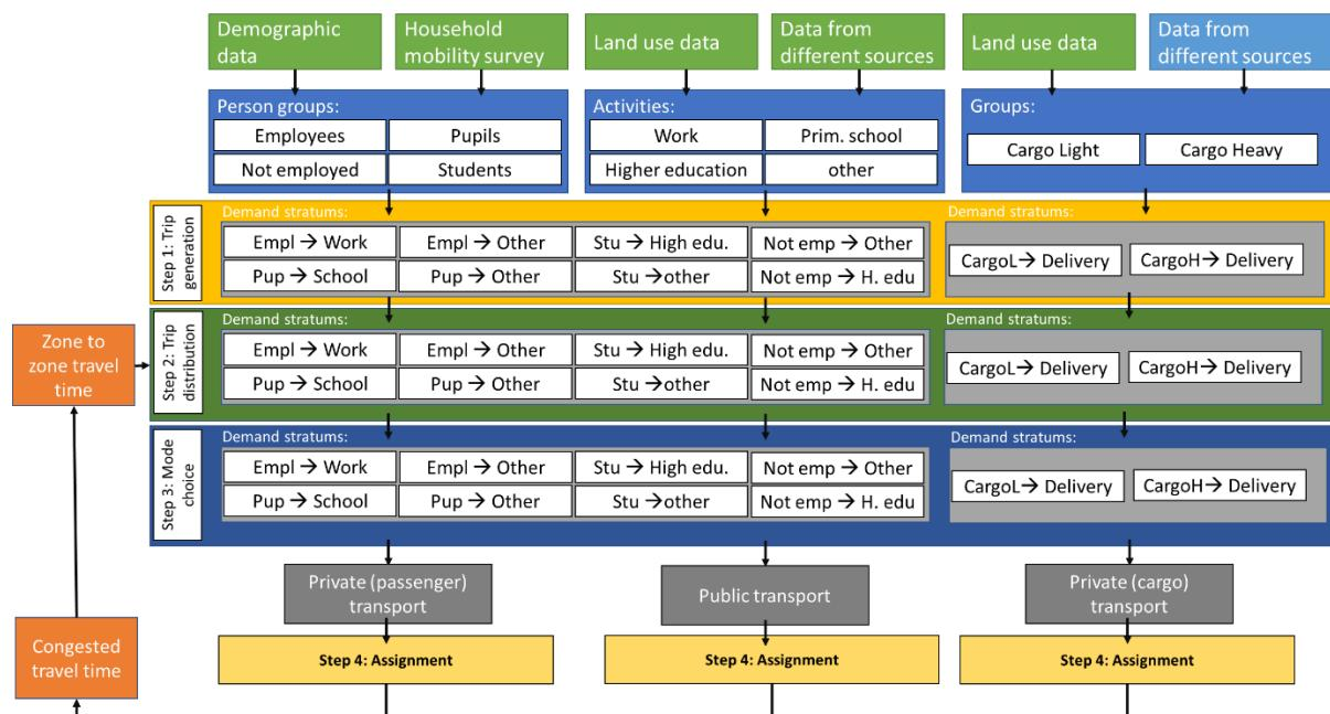
**Figure 11. Schematic workflow adopted in the project**
